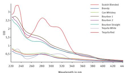
Fig. 2: UV-Visible fingerprint profiles of white and colored classes of distilled spirits.
