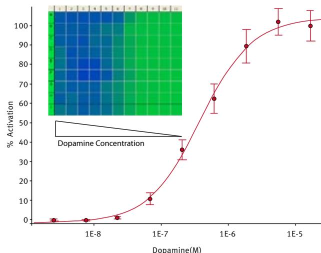
**Fig. 4:** Decreasing amounts of dopamine, a D1 agonist, (9 replicates) were added to Tango™ D1-bla U2OS cells (inset, columns 1-10) and the percent activation was plotted as a 4-parameter fit (negative control in column 11 was used as 0%). The PHERAstar FS' direct optic bottom reading, dual emission detection and orbital averaging (2 mm) were used.
