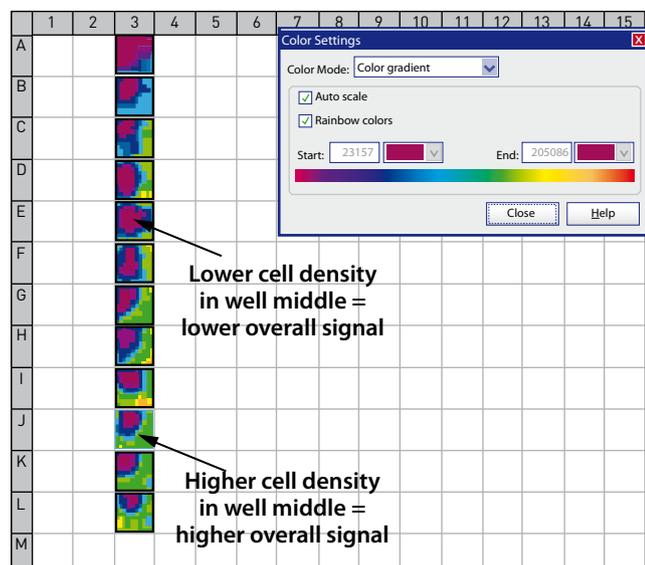
**Fig. 3:** Bottom reading high resolution cell layer scanning (10x10 matrix) shows the uneven distribution of HEK cells in each well. Samples with higher cell density in the middle of the well gave a more robust calcium response than lower density wells.
