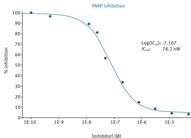
**Fig. 5:** Dose-response curve for inhibition of a PARP-family enzyme with a clinical PARP inhibitor (Olaparib).
