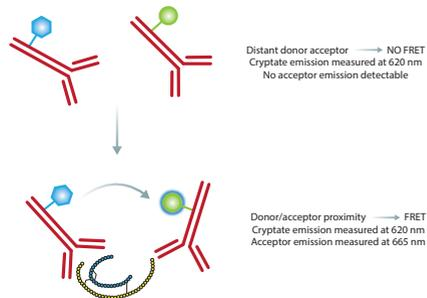
**Fig. 2:** Principle of the HTRF insulin assay. In the absence of insulin no FRET is occurring and only the donor will give a signal. The binding of both antibodies to insulin results in physical proximity, FRET occurs and acceptor emission can be detected. Ratiometric measurements reduce well to well variation.
