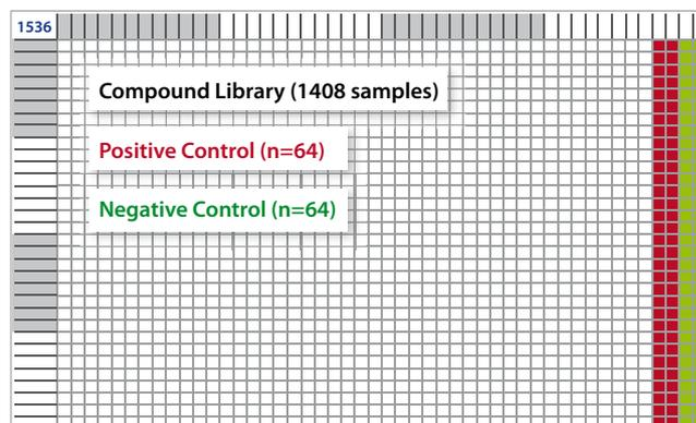
Fig. 3: 1536-well microplate layout
