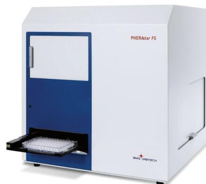
Fig. 1: PHERAstar FS microplate reader from BMG LABTECH
