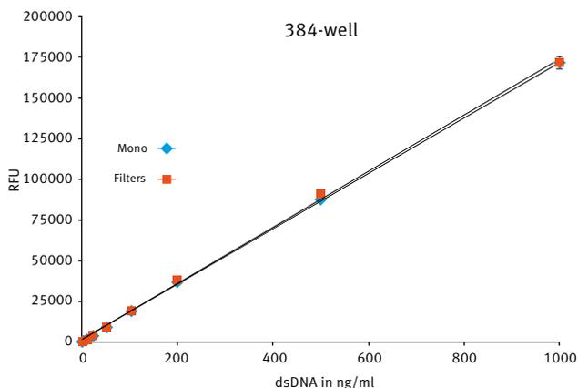
**Fig. 4:** PicoGreen<sup>®</sup> assay comparison using either filters (red) or LVF Monochromators<sup>™</sup> (blue) in 384-well format. The final volume in the well was 20  $\mu$ l.
