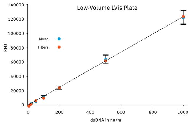
**Fig. 5:** PicoGreen<sup>®</sup> assay comparison using either filters or LVF Monochromators<sup>™</sup> in the LVIS Plate. The final volume in the well was 2  $\mu$ l.
