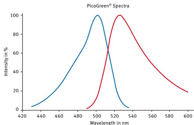
**Fig. 2:** Spectral scan of PicoGreen® reagent bound to DNA. The excitation scan (blue line) was recorded between 400 and 540 nm with a fixed emission wavelength at 550 nm. The emission was scanned between 490 and 600 nm (red line) while a fixed excitation wavelength of 460 nm was used.
