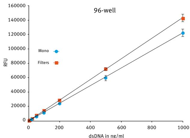
**Fig. 3:** PicoGreen<sup>®</sup> assay comparison using either filters (red) or LVF Monochromators<sup>™</sup> (blue) in 96-well format. The final volume in the well was 200  $\mu$ l.
