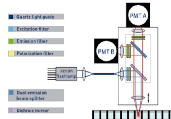
**Fig. 2:** New optical design of the PHERAstar
