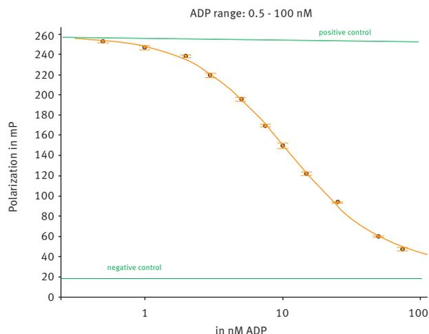
Fig. 4: 100 nM ADP/ATP standard curve measured on the CLARIOstar®
