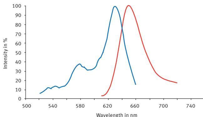
Fig. 3: ADP Alexa633 tracer from Bellbrook Labs Transcreener<sup>®</sup> ADP<sup>2</sup> assay was scanned on the CLARIOstar<sup>®</sup> using LVF Monochromator. The excitation of tracer was scanned between 520 and 660 nm, a constant emission wavelength of 690 nm was used. The emission was scanned between 610 and 720 nm at a fixed excitation wavelength of 580 nm.
