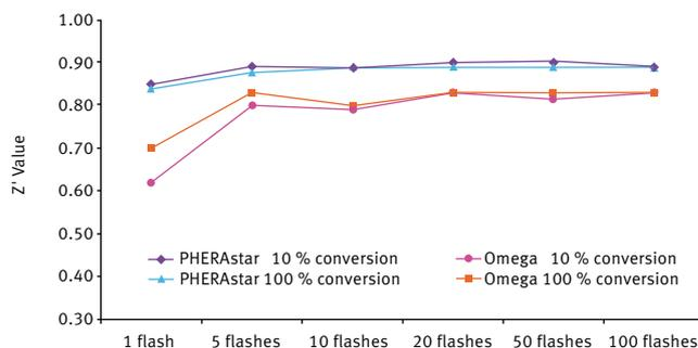
**Fig. 5:** Z' values obtained with the PHERAstar and Omega are dependent on the number of flashes. For the Z' calculation at least 20 replicates of ADP or ATP dilution were used.
