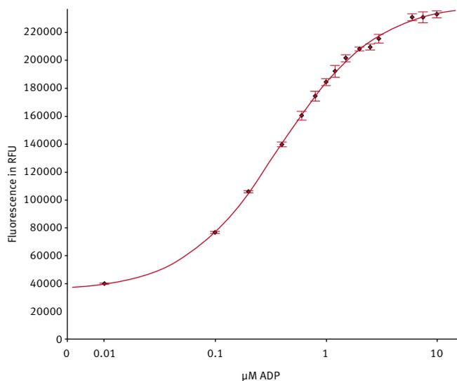
**Fig. 3:** 10  $\mu\text{M}$  ADP standard curve measured in 5 replicates using a PHERAstar Plus in 384 well format (20  $\mu\text{L}$ ). The concentration of 0  $\mu\text{M}$  ADP was set to 0.01  $\mu\text{M}$  to allow logarithmic scaling.
