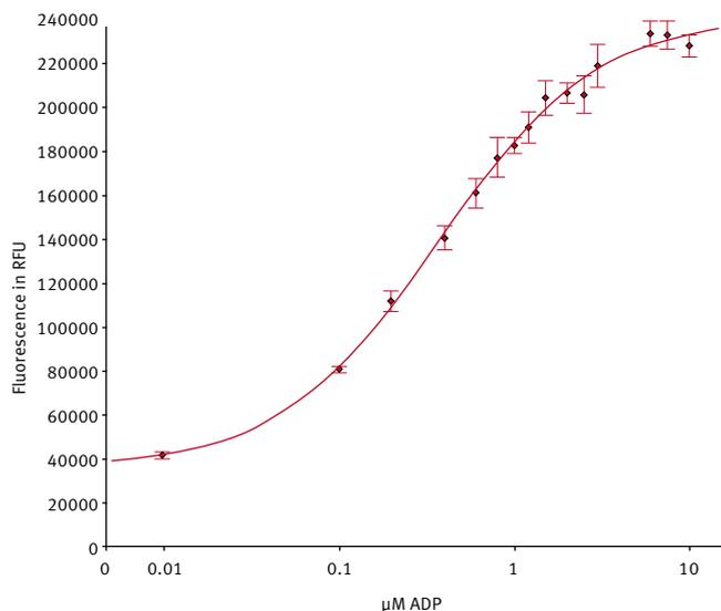
**Fig. 4:** 10  $\mu\text{M}$  ADP standard curve measured in 5 replicates using a POLARstar Omega in 384 well format (20  $\mu\text{L}$ ). The concentration of 0  $\mu\text{M}$  ADP was set to 0.01  $\mu\text{M}$  to allow logarithmic scaling.
