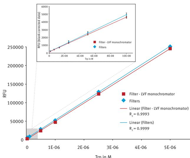
**Fig. 4:** Tryptophan linearity range measurements using either a combination of filter and LVF monochromator or just filters. The insert zooms into the low nM concentration range.
